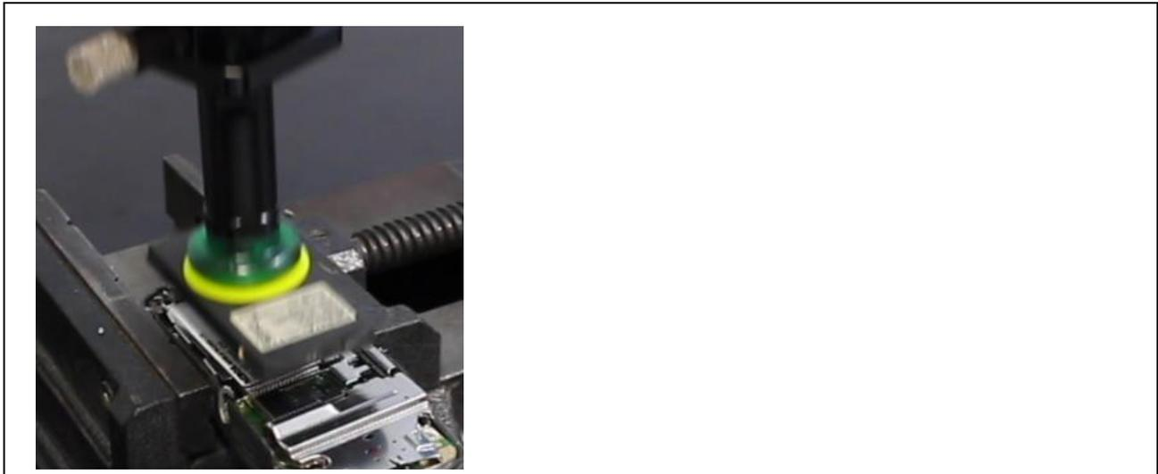
Figure 10: Withdrawal of a battery for an opened MPH by a suction cup
