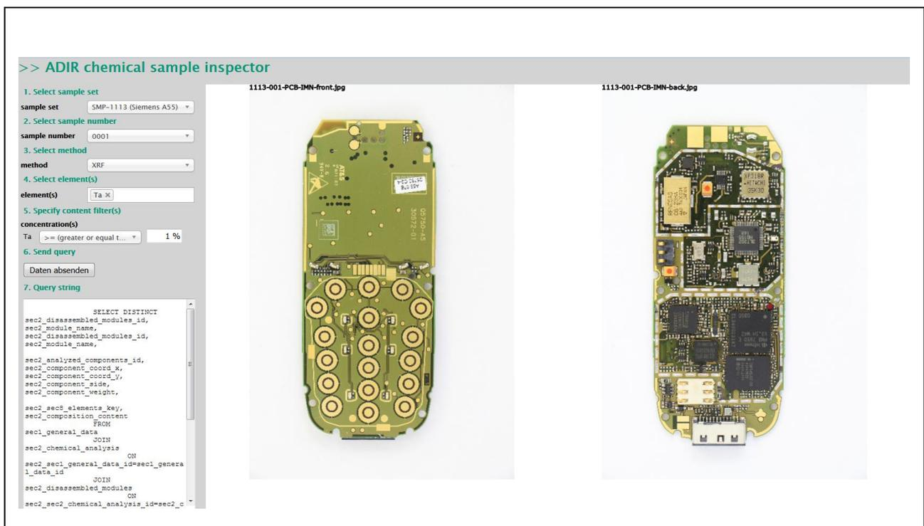
Figure 8: Screen shot of a query at the ADIR data base. High-resolution images of the front and backside of the PCB from the MPH model Siemens A55 are displayed. By a data base query (top left) compositional data with respect to e.g. tantalum are selected. In the shown example electronic components on the PCB are marked by a red dot where the tantalum content is greater or equal 1 %
