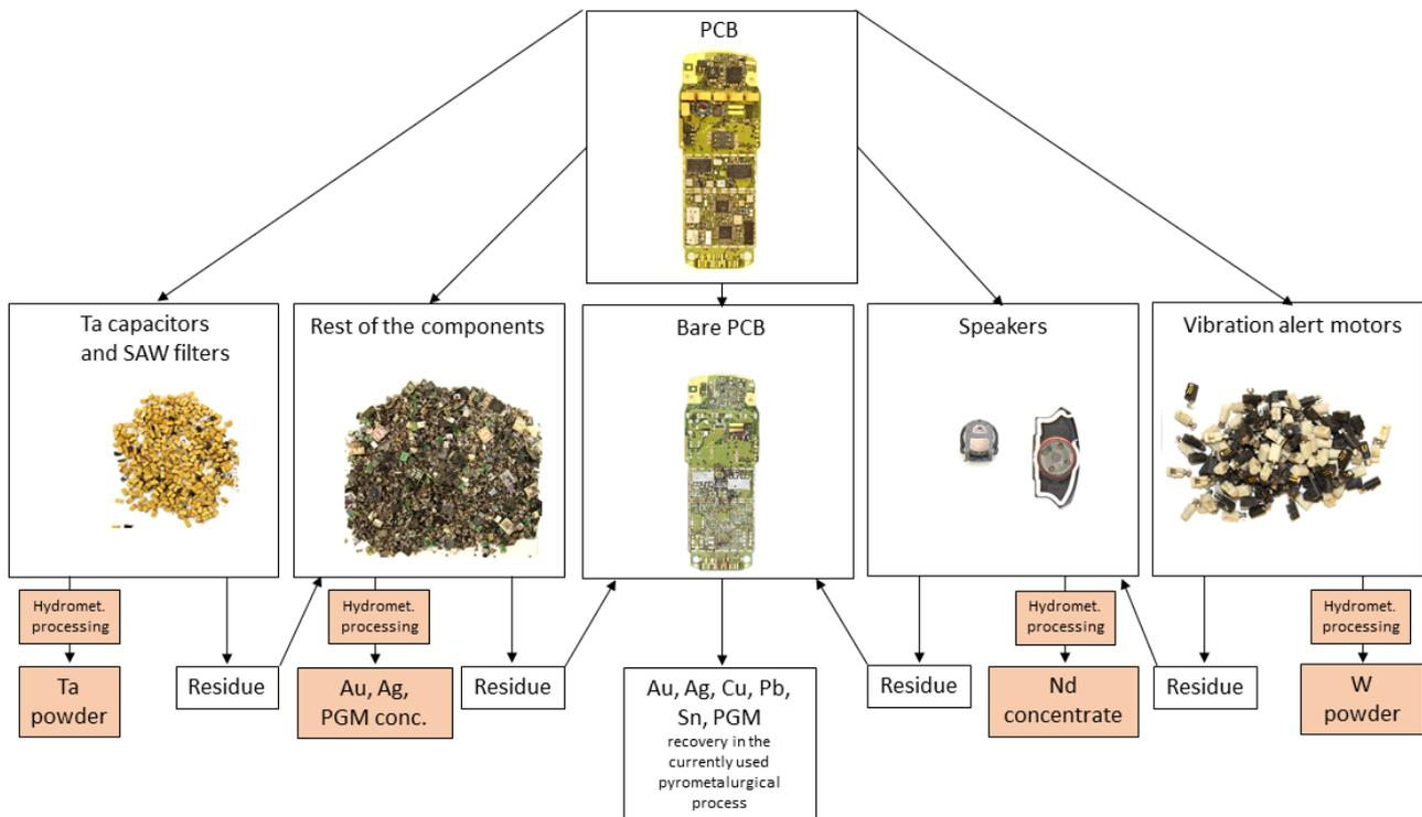
Figure 14: General overview of distribution of fractions and flow of processing streams with marked hydro-metallurgical processes
