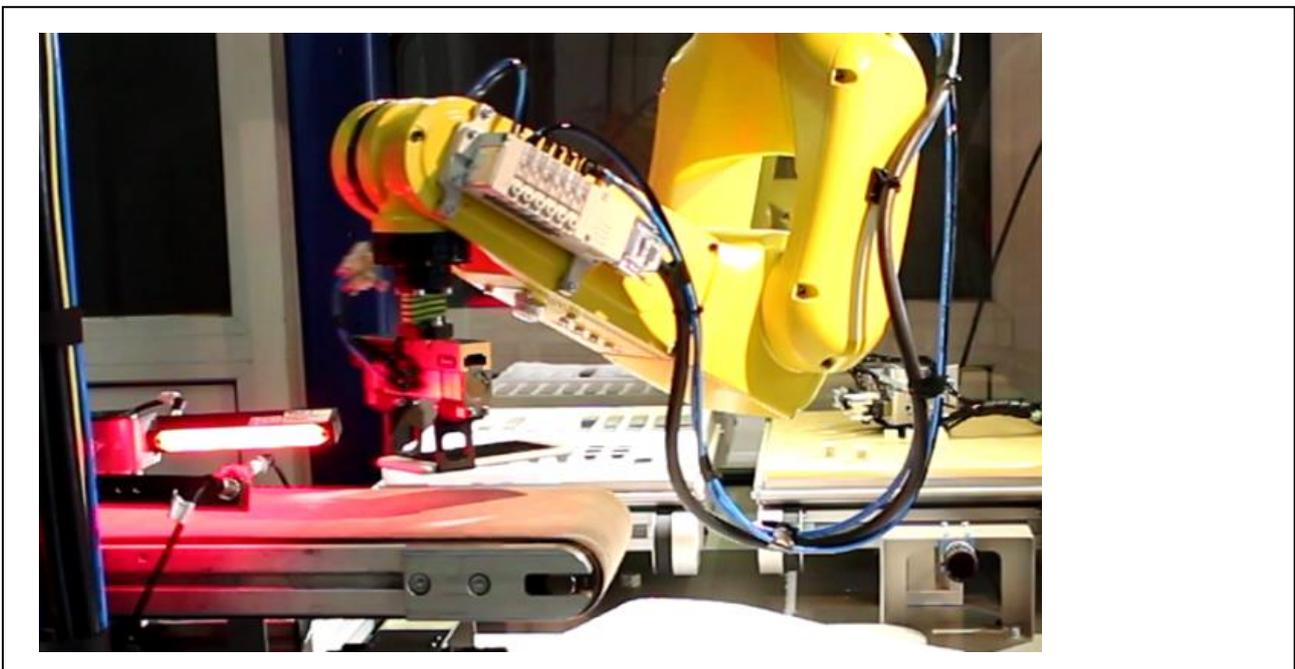
Figure 9: A singularized MPH transported on a belt conveyor, is first identified by a camera (see illumination above the conveyor) and then picked by a robot to transport the MPH to a clamping station for mechanical processing to open the casing to get access to the interior parts
