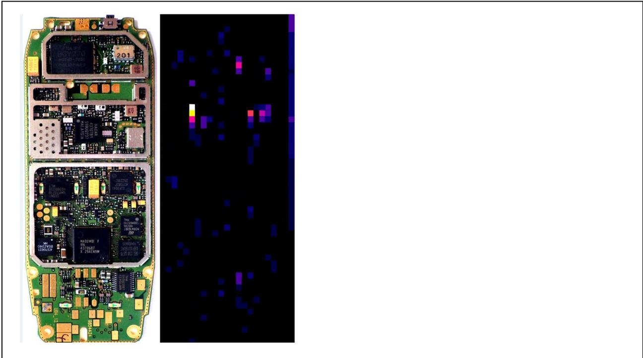
Figure 12: Left: photograph of the front side of a MPH, right: raster scan by laser-induced breakdown spectroscopy showing in false colors a chemical image of spectroscopic signatures of tantalum. An overlay of geometric-2D-image and chemical-2D-image yields the identified valuable components
