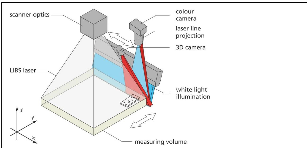
Figure 11: Principal set-up of machine II of the ADIR demonstrator. The PCB to be measured are positioned in a measuring volume. By a relative movement of a 2D- and a 3D-camera high resolution images of the PCB are taken. With a scanner optics a laser beam is then scanned to selected electronic components to measure a chemical information (LIBS)
