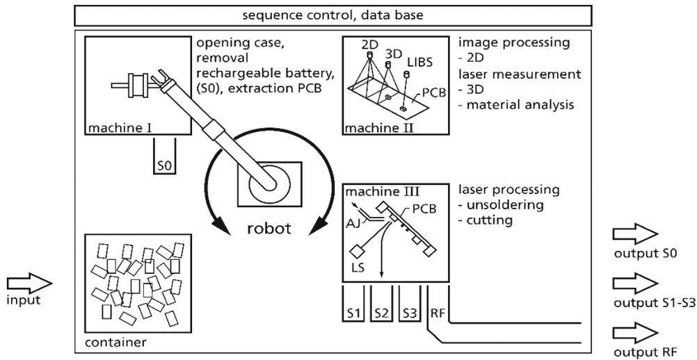
Figure 6: Concept of the ADIR demonstrator. A robot and a manipulator are picking single objects from the input stream and feed sequentially the machines I, II and III for selective disassembly of mobile phones and printed circuit boards (PCB)
