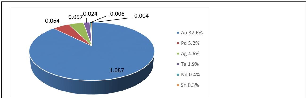
Figure 7: Pie chart of the average Euro-shares of the six most valuable target elements based on an analysis of the extracted electronic components from 13 MPHs (i.e. the values refer to the electronic components only and are given per PCB of a MPH). On the right side the average percentage shares are shown
