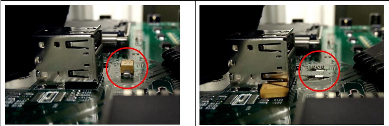
Figure 13: Left: snap shot of video sequence showing a tantalum capacitor to be desoldered (red circle), right: some tenths of a second later, the capacitor is desoldered and can be seen just left of the red circle
